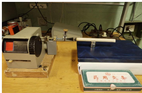
Fig.1. Photo of the input part of the RS and placement of moxa-rolls for measuring EMR in the millimeter range.
