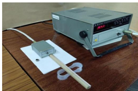
Fig. 2. Photo of the stand for evaluating the power of IR radiation of smoldering moxa rolls.
